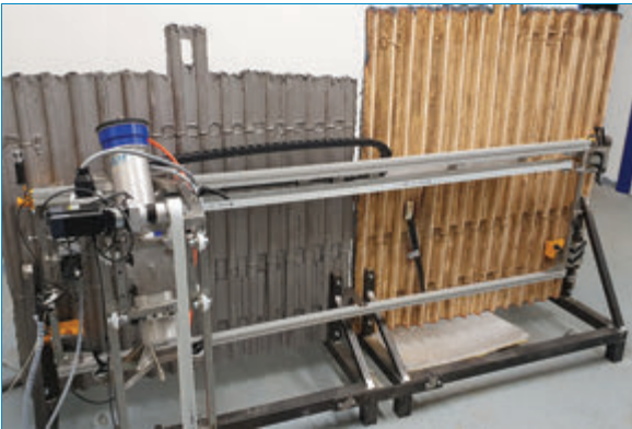
EXPERIMENTAL DR MANIPULATOR FOR TESTING OF PITTING CORROSION
