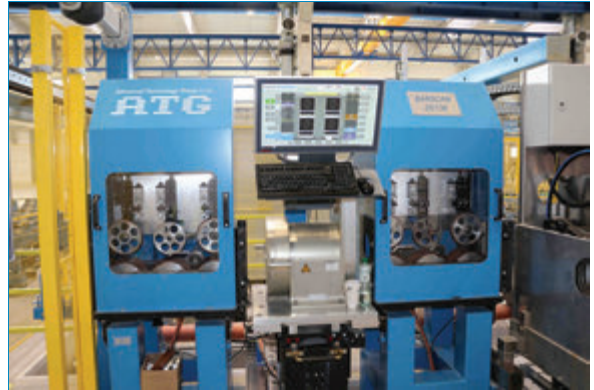
ET/UT BARSCAN 25-130 SYSTEM (AUTOMOTIVE) – ALUMINUM BARS
